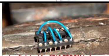
plug finished for 2716 EPROM before being dumped in black 2K-epoxyglue
